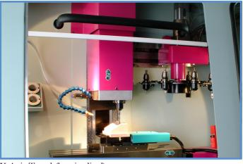
X Axis Travel (longitudinal) 304mm 157mm Y Axis travel (cross) Z Axis travel (vertical) 213mm Table Area 505 x 135mm Spindle to Table 260mm Centre Line of Spindle to Column 155mm Table to Column 5 to 162mm Tee Slots 3 x 10mm x 50mm Centres. Spindle motor 1.26kw Spindle speed 200 - 4000 rpm 110/220/240 V 1 Phase Electrics
