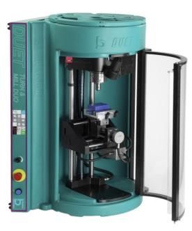
Slant-bed configuration in lathe mode.
