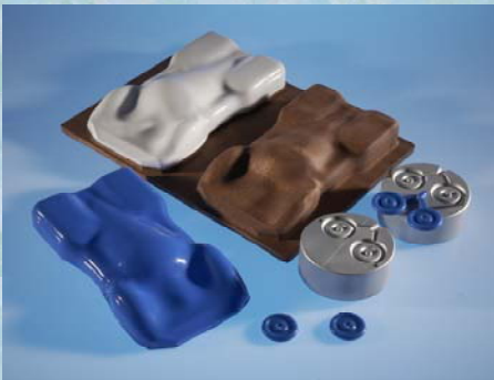
2½D Profiling and Blind Pocketing
